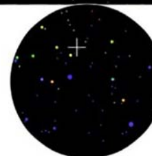
Figure 3.10 Electron- (a) and muon (b)-like neutrino interaction visible as single Cherenkov rings. The colors indicate the photon timing and the size of the dots shows the registered intensities in each photomultiplier. Reconstructed energies are 571 and 466 MeV, respectively. The distribution of fired photomultipliers is sharper for the muon-like event. Source: Kajita 2010 [143]. Reproduced with permission of The Japan Academy.
